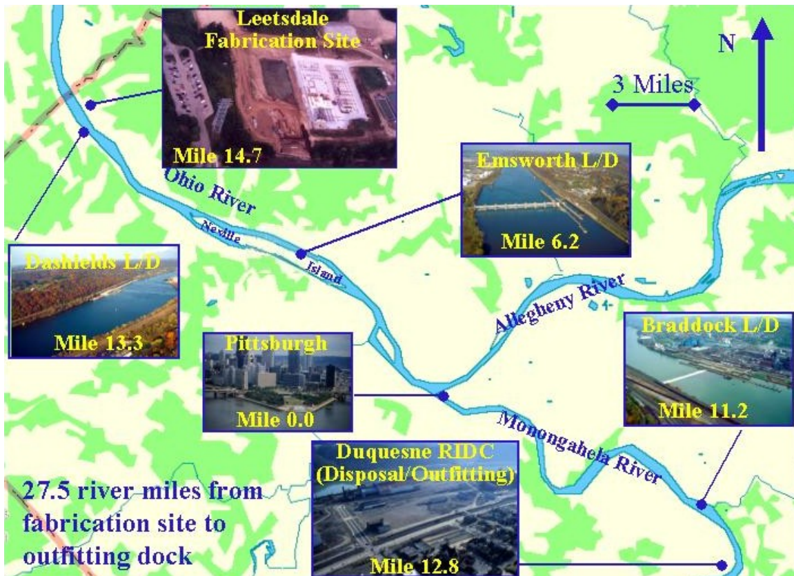
b. River miles from fabrication site to outfitting dock Figure C-12. Segment transport of Braddock Dam
